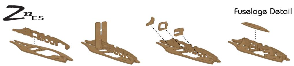
Step 13 - With the Vertical Spine on a flat surface, fit the right Horizontal Spine. Use the alignment tool, and tack in place // Fit the Struts by angling them in, top (long) tabs first, then rotating them down to the holes in the Vertical Spine. Tack in place // Fit the Drive Plate, arrow facing up. Tack in place
