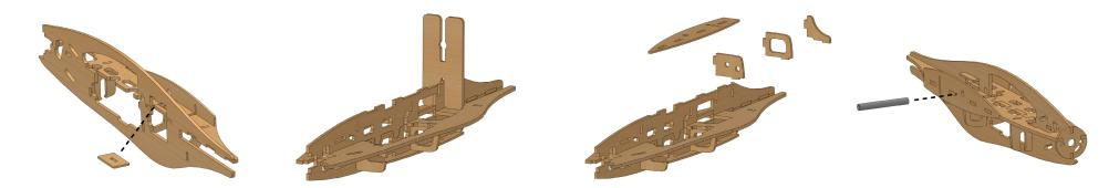
Step 14 - Fit the Servo Stop Plate. Square it up and tack in place // Fit the left Horz. Spine using the tool. Tack in place // Fit the remaining Struts and Drive Plate, squaring them up, and tacking in place // Insert the short aluminum Pivot tube into the assembly and center it up
