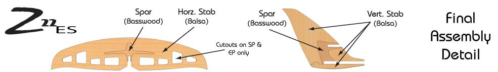
Step 16 - Fit the Spar into the Horizontal Stab, and press adhesive into the gap // Position the balsa Vertical Stab parts around the basswood Vertical Spar. Pin the perimeter, and press adhesive into the gaps // Sand the parts on a sheet of 320 grit on a flat surface to flush the basswood to balsa
