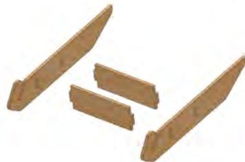
Assemble the tail jig with GAP. Use the Right Angle tool to square it up. If it's not flat, squared and near perfect, the tail will be out of alignment as well.
