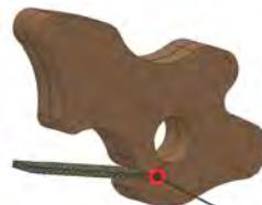
Fit the G-10 Spring Strip into the slot in the Latch Plate. Align and square up, then CA in place.
