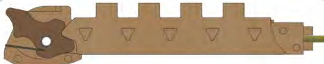
The function is fairly simple. The Latch Plate is spring loaded to lightly grip the Tail Blades. Pushing the Latch down, partially ejects the blades.
