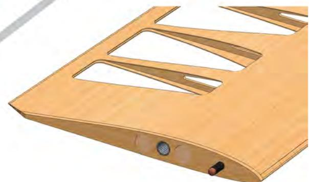
Allow the silicon to fully cure, then twist the Roller to free it. Turn it a few times to work it free from any residual adhesive.
