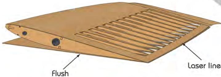
Lay the assembly on top of the Top Wing Skin. Note the laser line inboard of the trailing edge. Bring the Bottom Wing Skin's trailing edge up to the laser line, and make sure the root edge of the skin is flush with Rib #1.
