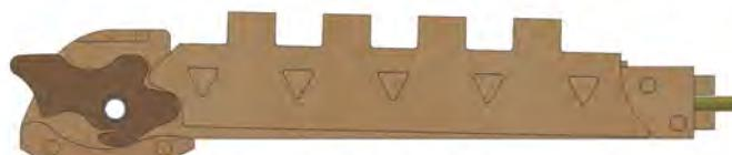
To load the Tail: Push down on the latch, and slide the Blades in, forward ends first. Pivot the tail-end down, while pushing forward, until you feel the Blades contacting the lower jaw of the Latch. And finally gently push the Tail down until the latch pops up.
