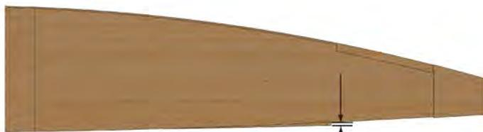
Refit the Bottom Cap cutout, so that the aft end is flush to the Bottom Cap, and the foreward end is pushed away from the surface the indicated distance.
