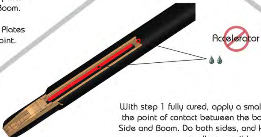
With step 1 fully cured, apply a small fillet of GAP at the point of contact between the bottom of the Box Side and Boom. Do both sides, and keep the fillet as small as possible.
