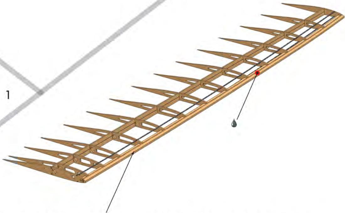
Sand both top and bottom of the Balsa Cap, to approximate an extended curve of the foil/rib section.
