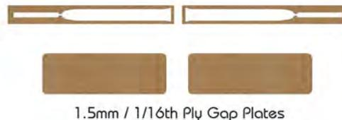
Lightly sand and test fit the two Gap Plates into the Cassette. They should be snug, without stressing the box. Wax both plates completely, then wipe any excess wax off.
